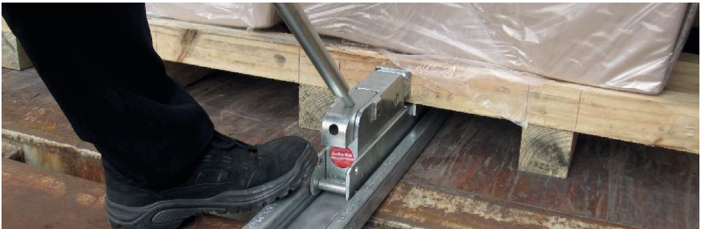
Example of the master skate positioned against the wooden slave pallet of the master skate positioned against the wooden slave pallet
