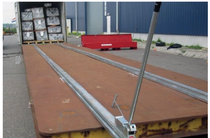
Example of a skate train for a 40ft one shot loading setup
