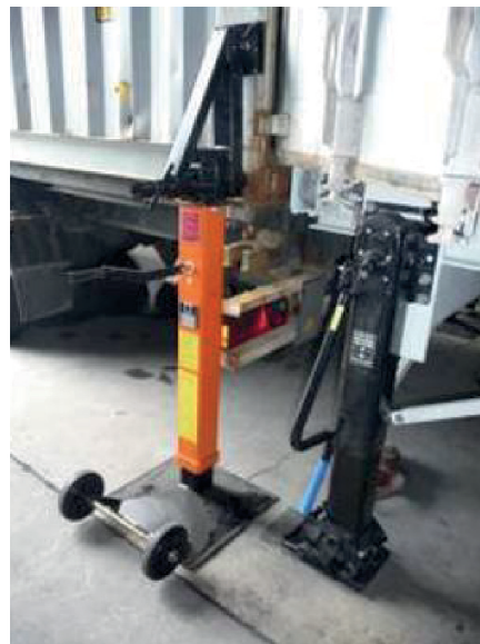
Examples of a chassis support placed underneath the chassis
