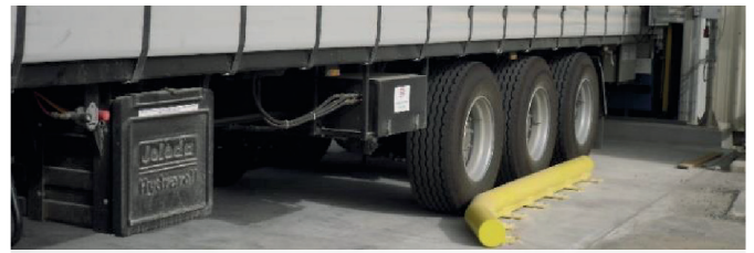
Example of semi-trailer positioned between wheel guides
