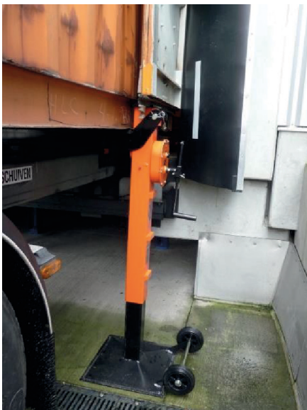
Examples of a chassis support placed underneath the chassis
